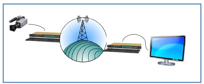
Both inserters must have a GPS antenna and be locked to GPS. The unit at the video source must be set to record time in the metadata (Metadata Write) and the destination end (where display is shown) must be set to read metadata (Metadata Read). At the destination, set the 6980G-HD to overlay the metadata time (see the command structure of the operations manual, or use the GUI supplied with the
